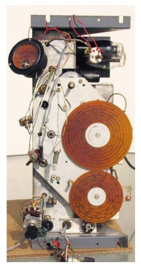
After final assembly, the bottom of the receiver shows the RF/Mixer/Oscillator coil assembly.
