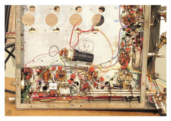
The rest of the IF strip and the Lamb noise limiter is shown here. Off to the right is the mode switch for the AVC and BFO. The original switch was lost, so a 2-wafer switch was configured to support the same functions.
