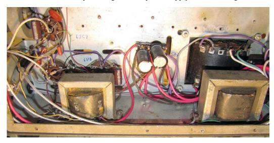
The electrolytic capacitors are replaced by units with high peak current rating on a newly-installed terminal strip to hold them. The audio stages are to the left with the 6SC7 first amplifier and phase splitter and the two 6V6 push-pull output amplifiers behind the output transformer.
