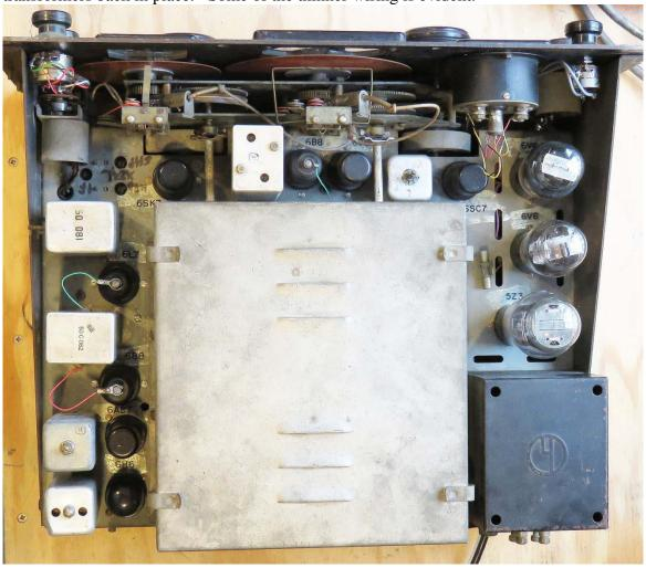
With the RF shield cover removed, the original metal octal tubes occupy the RF section, oscillator at
