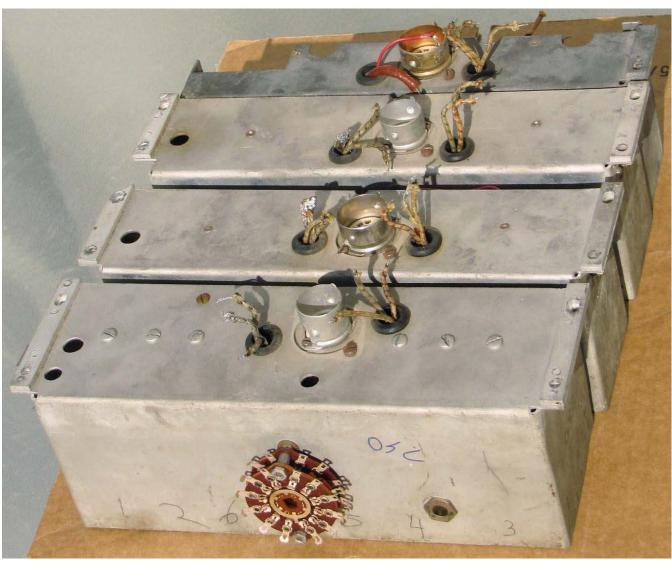
The miniature tube sockets are removed and the original octal sockets reinstalled. The original wafer switch at the front of the oscillator module has been lost. It controlled the IF gain separately for each band, as well as the RF AVC action for each band. New switch sections were found and configured to support these functions.
