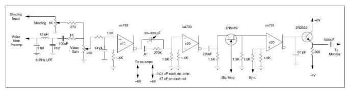
The voltage gain per stage is adjusted with external gain adjust resistors to be between 10 and 20.
