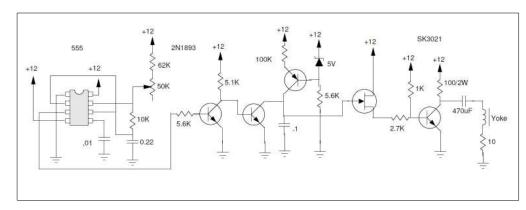
current source supplies the constant current, producing a linear ramp on the 0.1 uF capacitor that is amplified by the FET-NPN Darlington that drives the horizontal yoke through a DC blocking capacitor. The output transistor is a SK3021 that can take a several hundred volt pulse on the collector, which is set on a heat sink. The only control is the 50K 10-turn screwdriver pot that sets the frequency.
