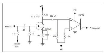
The op-amp has both inverting and non-inverting inputs, and inverting and non-inverting outputs, which is very useful in determining the proper polarity of the video. The voltage from the iconoscope mosaic is positive-going for black, and the video polarity out of the video chain provides a negative-going black signal.
