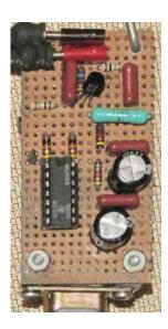
The preamp configuration chosen for now uses an NTE-312 depletion-mode NPN J-FET in common source configuration with a 1K drain resistor. This FET is a VHF amplifier with a 10 dB power gain at 400 MHz with a 2 dB noise figure at 100 MHz. Even with high-peaking in the video amplifier circuit, the amplifier noise level is acceptably low.
