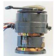
Knowing the rigidity of a 1 kV electron beam and the deflection angle of  $\pm 0.3$  radians, the peak current through the coil could be calculated, which is 100-200 mA, depending on the direction of deflection. A circuit simulation determined the voltage waveforms required, which amounted to a 500 volt pulse for the horizontal deflection coil. The vertical coil required a combination of pulse and sawtooth waveform of about 2 volts. Each current waveform is monitored by
