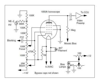
resistor string drains 2 mA and contains two potentiometers for focus and beam current, on HV standoffs for safety, and indicator lamps for filament (incandescent) and HV (neon) with green and red jewels.
