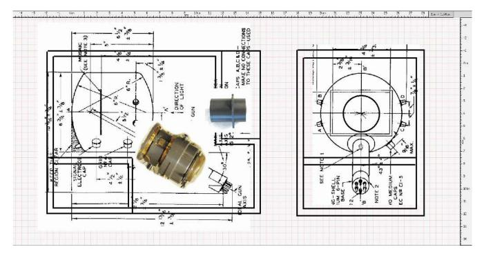
The entire case is Faraday-shielded with a copper screen completely lining the case, except for the lens opening. All the sections of the screen are connected together, and contact is made to the screen on the removable side through four banana-plug mounting points.
