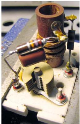
These individual coil modules are held onto the turret with small clips. Don't let these get loose and fly off!
