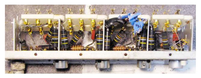
Here, the BBs have been replaced with "orange drop" capacitors of the same value.
