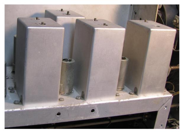
The covers come off easily upward, exposing the coil sets and the BBs beneath them.
