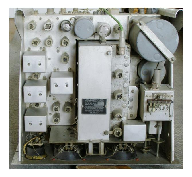
Many of the coupling and bypass capacitors in this receiver are the so-called "Black Beauties" (BBs) that over the last 60 years have seriously deteriorated by becoming electrically leaky with significant changes in capacitance.
