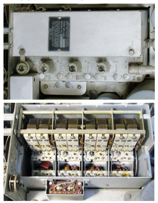
Here, the module containing the two RF stages, the mixer and oscillator has been removed from the RF deck, showing the top of the bandswitch turret. The multi-gang tuning capacitor is at the top, and the power supply tie points are in the small shielded compartment at the bottom.
