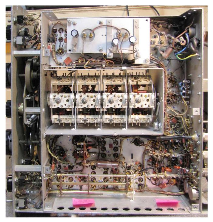
Here are all the capacitors removed, including a few from previous recapping.
