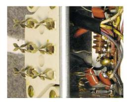
The Black Beauty capacitors are visible in the RF module. The first RF stage is at left, and the oscillator is at right. The disconnected power wires are identified with the blue tags.
