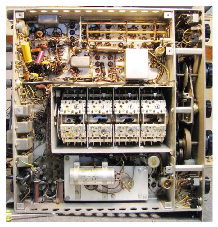
With the bottom shield removed, the turret is visible.
