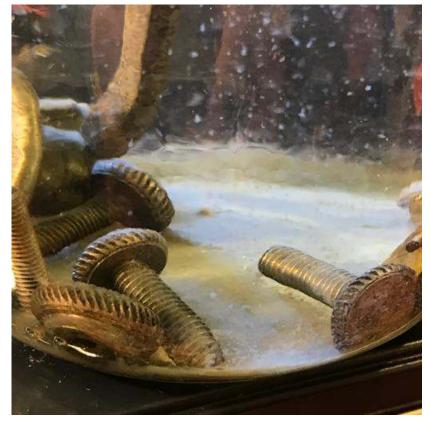
Corrosion precipitates off and settles at the bottom of the glass jar.
