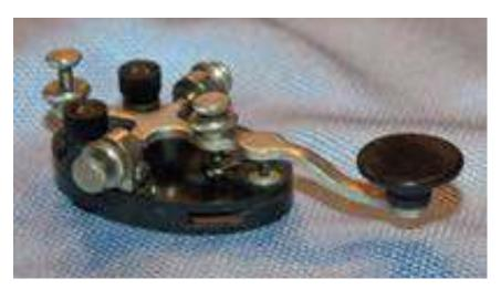
CLT-26012B is a nearly identical key with an insulated knob. Like the Bunnell key, it is a World War Two era open circuit key. Lundquist Tool & Manufacturing Co., of Worcester, Mass. fulfilled this "B" contract. (A closed circuit landline key uses a horizontal lever to keep the circuit closed except when keyed, in order to always receive messages on the circuit).
