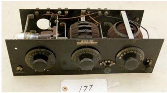
177. AMRAD / 3730 1923; TRF broadcast tuner; has tube; no cabinet
