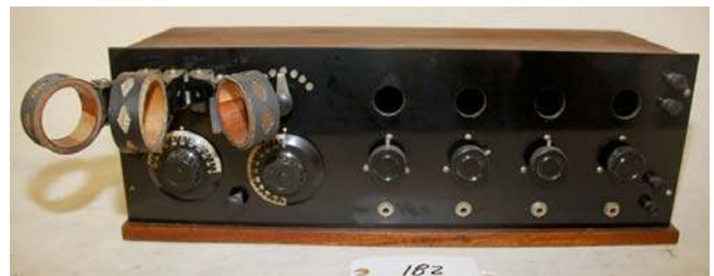
182. Homebrew / . Early 1920s; regenerative; has DeForest type coils; no tubes
