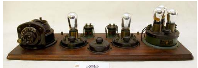
180. Atwater Kent / 4066 aka Model 7 1923; TRF; 5-tube breadboard
