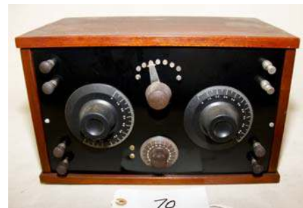
70. Homebrew / . Mid 1920s; regenerative; has display which is or similar to Moorhead electron relay
