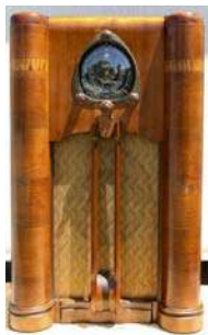
171. Zenith / 9S232 1938; BC/SW; 9-tube 3-band Shutter Dial; Recapped; working well.
