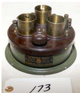
173. Atwater Kent / TA 1922; 3-tube detector and 2-stage amplifier component
