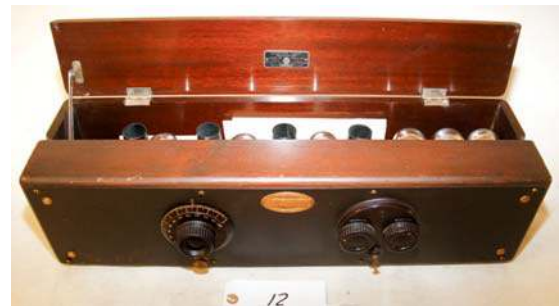
12. Atwater Kent / 32 1926; TRF; has tubes
