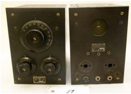
17. Westinghouse / RA & DA 1921; regenerative; has tubes; DA possibly modified for Military
