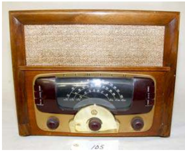
105. Zenith / 8H861/8E20 1948-49; Broadcast band and both FM bands (new and old); works
