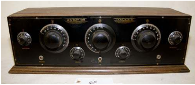
65. AC Dayton / Type XL-5 1924-25; TRF; no tubes
