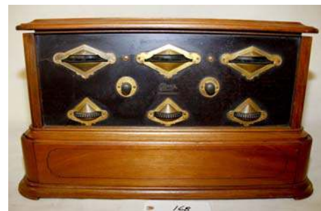
168. Grebe / MU-1 Synchronphase 1926; TRF; has chain drive; no tubes; has added cabinet base for battery storage
