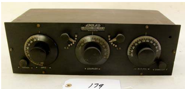
179. AMRAD / 3475 1923; TRF broadcast tuner
