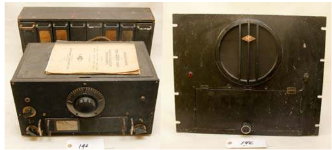
146. National / HRO Circa 1934; Multiband receiver with amplifier; has coil sets in a case
