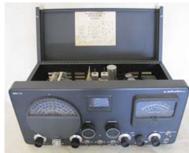
28. Hallicrafters / S-76 1951-55; 4-band communications receiver; working
