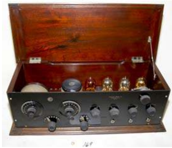
169. Simplex / Type-RF 1923-25; TRF; has display tubes which are or similar to Moorhead electron relays
