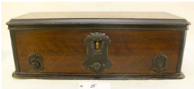
5. Radiola / 60 1928; BC; superheterdyne; has tubes
