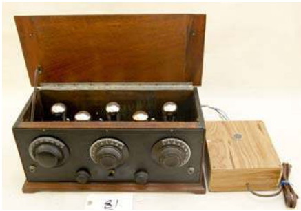
81. Freshman Masterpiece / . 1924; TRF; has tubes; includes homemade power supply
