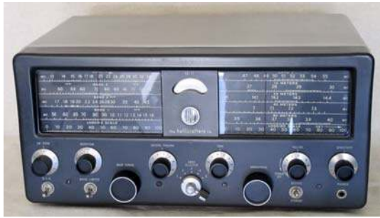
73. Hallicrafters / SX-71B Early 1950s; 5-band communications receiver; working
