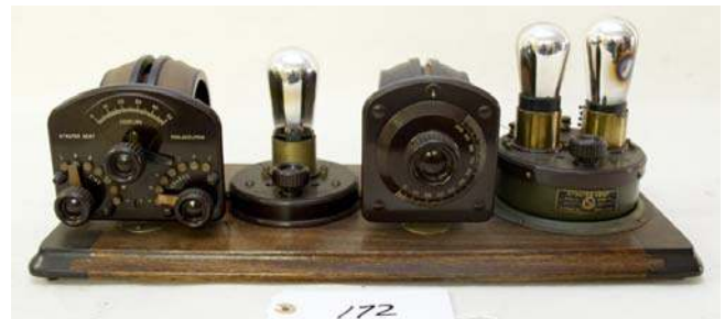
172. Atwater Kent / 3975 ? Circa 1922; TRF; 3-tube breadboard
