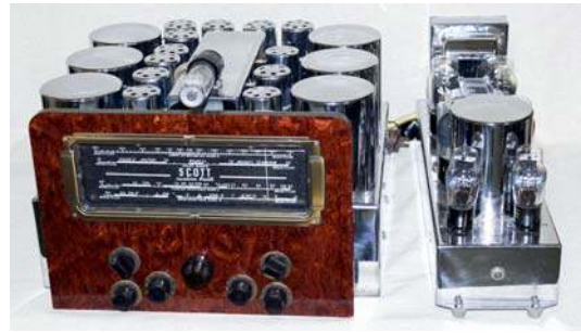
154. Scott / Phantom 1938; receiver and amplifier chassis; 19 tubes; BC/SW; no speaker; believed to be working
