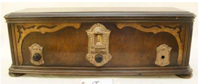
19. Brunswick / 5NO 1928; Superheterodyne; broadcast band; has tubes
