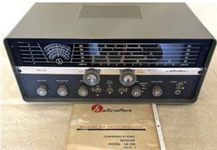
51. Hallicrafters / S-108 1959; VHF/HF communications receiver; working
