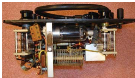
RS-1 transmitter interior (1)
