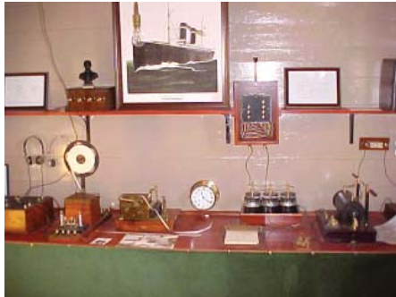
Fig. 4. A wireless telegraphy shore station of the first decade of the 20 th century; a spark gap on an induction coil to the right, Leyden jar condensers to the left, clock center, ink for recording received signals and in front of it, a coherer detector, and to the left of the coherer, the tuner for reception. This is a reconstruction of the Marconi station at Lizard Point, Cornwall, UK; curator David Barlow. (Photo Bart Lee, 2005).
