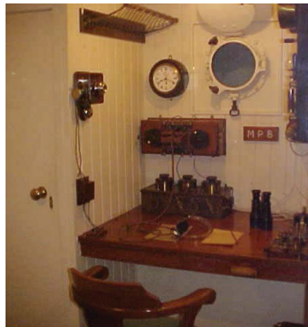
Fig. 5. A Marconi ship station (Empress of Britain, callsign MPB), tuner to the left, as reconstructed at the British Museum. (Photo Bart Lee, 2002)
